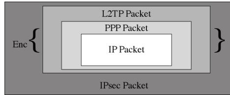
An outgoing IP packet is encapsulated in a PPP packet. This PPP packet is encapsulated in a L2TP packet. Again, this encapsulation does not make any sense, but it is declared 'Standard' from Microsoft. The resulting L2TP packet is finally encrypted (Enc { }) by the IPsec stack, the IPsec headers and trailers are added, and the resulting ESP packet leaves the network interface.
